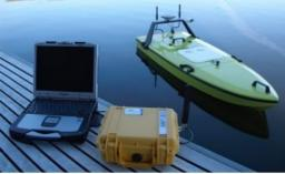
With a purposeful-looking remotely operated hydrographic survey boat package, CEE HydroSystems USA has added a factory-option USV to its shallow-water bathymetry product line. The survey vessel is 1.9m and equipped with a singlebeam echosounder. The key to the CEE approach is to bring all components together; instead of multiple components cabled and connected, the CEE-USV has a single data module presenting a simple user interface.
