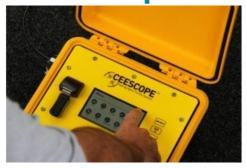
CEE HydroSystems has released an 'all in one' hydrographic single beam echo sounder survey system, designed for users wishing to obtain the benefits of precise multiconstellation GNSS positioning through the Hemisphere Atlas L-Band subscription service. With the Hemisphere GNSS P326 Eclipse OEM receiver installed inside the waterproof CEESCOPE enclosure, the CEE package offers a scalable approach combining dual frequency GNSS with the world-wide Atlas L-Band correction service.
