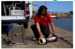
Sonardyne's 6G (Sixth Generation) acoustic positioning technology was demonstrated to industry professionals during in-water demonstrations in Stonehaven Harbour on the east coast of Scotland. For three days last week, a Long BaseLine (LBL) positioning network of six Compatt 6 transponders was set up against the walls of the harbour, in depths of as little as two metres. A Dunker 6 LBL and telemetry transceiver was then used to perform an array calibration and collect acoustic range data.
