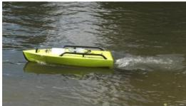
The ARCboat Lite is a portable and compact version of HR Wallingford's award-winning remote-controlled survey vessel, the ARCboat. Weighing only 15kg and just 1.3m long, the ARCboat Lite can be carried and deployed by a single person and easily fits inside the boot of a typical family hatchback. It can operate in flows of up to 2.5m/s, in water as shallow as 22cm, and it costs less than the larger ARCboat.
