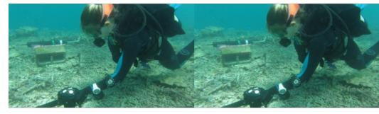
Researchers at the Heron Island Research Station in Australia are using a Nortek velocimeter to determine how much hydrodynamic energy it takes to move "coral rubble", the skeletons of corals broken apart by bleaching or storm events in the ocean. Fortunately, researchers have found that stabilizing rubble can be an effective technique for coral reef recovery.
