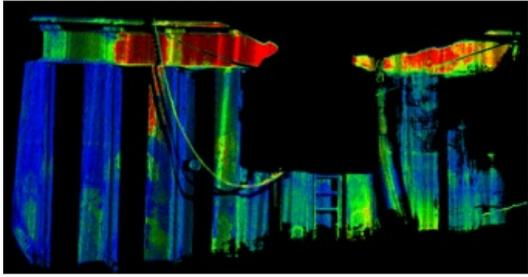
Locating and investigating retaining wall deterioration in its early stages is critical for ensuring the protection of the coastline and for avoiding extensive repairs or costly replacement. ADUS DeepOcean recently deployed the 2G Robotics ULS 500 in profile mode to continuously scan and generate a high-resolution 3D model of a corrugated wall. The high resolution of the scans provided a detailed understanding of the wall's condition and enabled signs of corrosion and wear to be easily detected.
