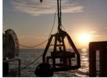
UK-based Coastline Surveys, which was contracted by Calegeo for an Alcatel Lucent cable burial assessment survey, recently broke its own water-depth record with its C-Pen40 seabed CPT system. After mobilising in Turkey, 44 tests were completed to full penetration across the 210km route between the landfalls. With a steep shelf on both sides, most of the CPTs were undertaken in water depths of over 1,000m and with a record depth of 1,250m being achieved successfully.
