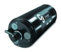
Turner Designs offers a Deep UV Optical Kit for their C3 Submersible Fluorometer which enables detection of refined oils and fuels. Recent developments in LED technology allow for excitation wavelengths down to 260nm. Using BTEX as the standard, the C3 is able to detect as low as 0.1ppm over a dynamic range >2500ppm.
