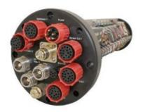
The MacArtney NEXUS MK VI is a HD video and multibeam sonar multiplexer that carries all signals over one single mode optical fibre via CWDM (Coarse Wavelength Division Multiplexing). As a frequently selected option, the multiplexer comes with integrated (P)ECL and 10/100 Ethernet cards. It is designed and built to be a rugged, efficient and versatile HD solution for interfacing a wealth of different sensors, equipment and subsea systems to over 3,000m.
