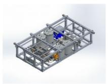
Chukar Waterjet, USA, introduces its SUB-JET 3000 subsea waterjet system for work class ROVs. Operable at depths up to 3,000m (10,000 feet), the SUB-JET 3000 cuts steel up to 250mm thick and blasts away coatings, corrosion and marine growth at pressures up to 3,900 bar. Because it is deployed with an ROV, the SUB-JET 3000 is less expensive than a standalone subsea waterjet system.
