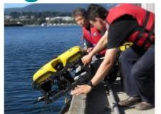
The Department of Fisheries and Oceans Canada in Manitoba will use a SEAMOR Marine Remotely Operated Vehicle (ROV) to inspect the High Arctic area which remains frozen year-round. The Chinook ROV will take part in research and evaluating ways to protect this special ecological region. The vehicle will also be used to conduct ecosystem identification and benthic surveys (underwater mapping of the seafloor) and inspection of first-year ice and multi-year ice.
