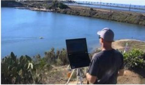
BioSonics and The Oceanscience Group (USA) have released a portable, remotely operated habitat-mapping survey boat, the Z-Boat 1800MX. A combination of Oceanscience's remote hydrographic survey boat and BioSonics' MX echosounder, the Z-Boat 1800MX allows researchers to obtain quantitative measurements of aquatic vegetation and substrate distribution without the expense and effort of launching a manned boat.
