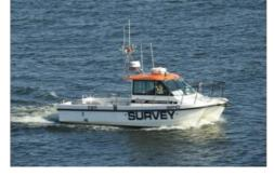
Underwater survey company Deep will upgrade one of its survey vessels with a Sea Machines SM300 autonomous control system. The Sea Machines system enables remote command of the vessel, including navigation and positioning, the control of on-board auxiliaries and sensors, and ship-to-shore data flow. The vessel, operating in multiple areas of the Wadden Sea, will be commanded by
