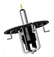
HydroBar is a hydrographic tool for calibrating survey echo sounders during field surveys. A real-time sound velocimeter is combined with a sonar target ( bar') and Windows-based software which can run on a PC in the background of Hypack, HydroPro or other hydrographic software.
