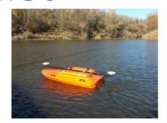
Seafloor Systems has successfully integrated and tested the Norbit iWBMSc (Integrated Wideband Multibeam Sonar, Compact) echosounder system with the EchoBoat-RCV remotely controlled survey vehicle. In addition to its ultra-compact form factor, the Norbit system features an integrated INS and sound velocity sensors, thus eliminating the need to install separate devices while greatly
