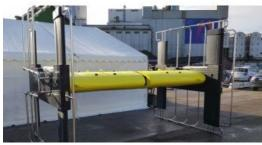
The EIVA ScanFish remotely operated towed vehicle (ROTV) is designed to function as a platform for subsea sensors. It comes with a maximum sensor payload of 50kg as standard, but the total payload capacity for the EIVA ScanFish is 350kg.
