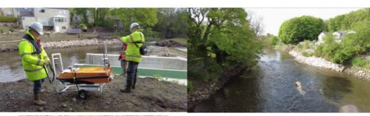
In early spring 2021, Storm Geomatics were approached by an existing client to carry out topographic and bathymetric surveys on the River Aire, in the village of Newlay, to the north-west of Leeds, Yorkshire, in the UK. The survey was required to provide information for local asset recovery works.
