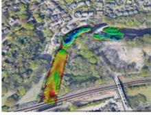
In the extremely shallow river, the system supplied by THURN Group, compromising the OceanAlpha SL40 Unmanned Survey Vessel (USV) equipped with a GeoSwath4 Interferometric Sonar and SBG Ekinox IMU, enabled Storm Geomatics to carry out a full bathymetric survey efficiently and safely in a difficult to access and fast-flowing section of the River Aire.
