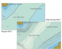
Germany-based SevenCs has released a brand new member of the ENC Tools family. ENC Bathymetry Plotter assists the producer of nautical charts in contour generation and helps to reduce the manual work. The contouring process is based on a shoal-biased Nautical Elevation Model and creates contour lines that have a smooth appearance and do not require any further generalisation.
