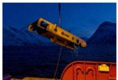
An AUV designed to carry out subsea environmental monitoring along predetermined tracks is being tested by Eni Norge. Together with its subsidiary Tecnomare, Eni Norge has completed the research and development project "CleanSea". The development of an AUV, carrying out sampling which is important as part of monitoring the marine environment, was one of the aims of the project.
