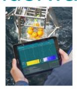
Leaks on offshore platforms present a hazard to the marine environment and human health. The monitoring system FlexMoT will detect irregularities and provide a warning system for disasters. The system was presented at this year's OCEANS'16 in Monterey. FlexMoT is an autonomous, flexible monitoring tool with two essential tasks: it works as a long-term monitoring system and it can be deployed at short notice in emergency situations.
