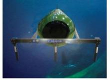
INNOVATUM, UK, has carried out successful testing, including autonomous operation of the Smartrak cable and pipeline tracking system on AUVs. This integration enables the AUV to navigate to the target cable or pipeline, follow it and measure position, including "Depth of Burial".
