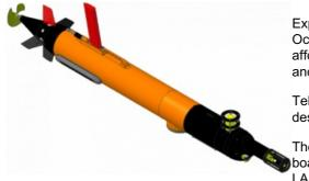
Explorer Doppler Velocity Logs (DVLs). They have been successfully integrated on OceanScan-MST's light autonomous underwater vehicle system (LAUV), which is an affordable and innovative one-man portable AUV that can be easily launched, operated and recovered with minimal setup.
