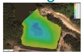
Eye4Software, The Netherlands, has announced that the latest version of its hydrographic survey package, Hydromagic version 5.2, has been released to the public. The main purpose of this software is to map the bottom of a river, reservoir or ocean in 3D, by using a (D)GPS or RTK positioning system combined with an echosounder or fishfinder.
