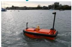
ASV engineers travelled to Tohoku University in Japan to hand over C-Stat 2, the first autonomous mobile station keeping buoy. Designed and developed by ASV, the buoy will be used by the university to help predict earthquakes off the Japanese coast.
