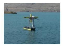
The newest aircraft carrier does not have acres of flight deck. In fact, it has no deck at all. Rather than carrying a crew of thousands, it sails without a soul on board. Yet the aircraft that it operates can fly much longer and further than anything based on a fleet leviathan. That aircraft is Aerovel's 20kg Flexrotor, which combines VTOL and a small footprint with a Hawaii-to-West Coast range. The carrier is a 4-metre skiff equipped to launch, retrieve and service the Flexrotor automatically.
