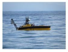
ASV Global and TerraSond have completed their first ever seabed cable route survey supported by an unmanned surface vehicle (USV). The survey route included various water depths and strong currents, while facing difficult wind and sea conditions in the Bering Sea offshore Alaska. The project was mobilised immediately following a 9,000km nautical charting survey by Terrasond, of which 4,750km (53%) were executed by an ASV Global C-Worker 5 autonomous surface vehicle (ASV).
