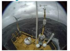
The EDP Inovação (EDPi) WindSentinel floating Lidar system has survived a major storm that ravaged the shores of Portugal near Viana do Castelo on 16 October 2014. Enduring gale force winds with gusts of over 90kmph and waves the size of three-storey buildings (10 metres high), the AXYS WindSentinel remained on-station and fully operational with 100% data availability.
