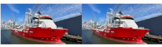
Fugro Quest, a vessel equipped with advanced deep-water technology, is the newest addition to Fugro's geotechnical vessel fleet. Fugro uses this type of vessel to determine the exact composition of the sea floor; the resulting data are essential to establish the optimal location and design of offshore developments such as wind farms.
