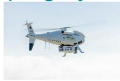
Fugro recently introduced its nextgeneration coastal mapping system, the Rapid Airborne Multibeam Mapping System (RAMMS 2.0), at the Hydro 2023 conference in Genoa, Italy. RAMMS 2.0, the world's only airborne Lidar system capable of delivering both full water column imaging and high-resolution bathymetry, is designed for precise mapping, monitoring and modelling of
