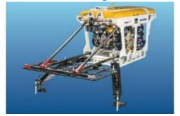
For the first time, a full pipeline survey spread has been fitted to a Saab Seaeye ROV in the shape of the Panther XT Plus. The innovation is to bring considerable savings in survey operating costs to operators when compared to deploying a 150hp hydraulic work-class vehicle for the task. Being acoustically quieter than a hydraulic vehicle, an electric ROV will also produce more accurate multi-beam sonar data.
