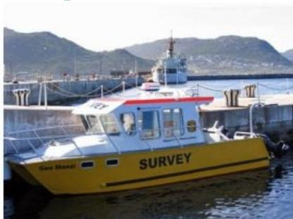
The Marine Geoscience Unit (MGU) of the Council for Geoscience recently launched its latest survey vessel, the SV Geo Manzi, in Simon's Town near Cape Town, South Africa. Geo Manzi (Zulu for Geology and Water) has an overall length of just under 9m, with a beam of 3.1m and a draught of ~ 0.6m and was built by Cape Town-based Veecraft Marine. She is powered by twin 4-stroke Suzuki outboard motors of 175HP each which allows her to reach transit speeds in excess of 35knots.
