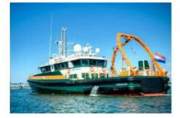
A technologically advanced vessel has been added to the Netherlands-based Geo Plus fleet, with the christening of the Geo Focus on 23 June 2012. She is a 35m diesel electric vessel, capable of sailing without the main engines at a speed of 10kn, thus reducing fuel and Nox. Geo Focus can operate 24/7 for a period of two weeks.
