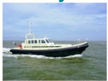
Geo Explorer is a 16.40m long, 5.20m wide fast survey vessel, capable of completing surveys in sea and shallow water. Equipped with multi-beam, she can fulfill a wide range of surveys in the 30 mile-zone in sea.
