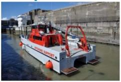
GEO.xyz, headquartered in Belgium, took delivery of its latest vessel, Geo Surveyor X, in October 2013. Designed to GEO.xyz's specifications, Geo Surveyor X is a 20-metre multi-purpose vessel fitted with the latest survey equipment including a hull-mounted multibeam system. It is able to carry out the full range of site and cable route surveys in a safe and efficient manner.
