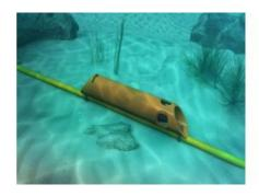
Sercel (France) has launched GeoTag, an acoustic positioning solution for seabed seismic acquisition. GeoTag can be used to accurately position all types of ocean bottom cable (obc), ocean bottom node and transition zone cable systems for seabed seismic surveys in water depths down to 500 metres.
