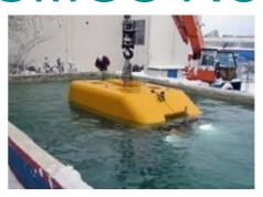
Amidst -3°C temperature and snow, ISE commenced trials and testing on the China Geological Survey ROV for its first test dive in the ISE pool. Named "Sea Lion", the ROV is an ISE HYSUB 130HP ROV scheduled for delivery in the first quarter of 2009. Sea Lion is the first ROV for Guangzhou Marine Geology Survey (GMGS), a division of China's Ministry of Land and Resources.
