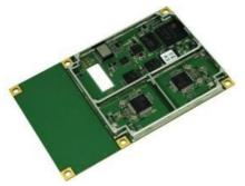
Canada-headquartered Hemisphere GNSS has launched its Crescent Vector H200 GNSS compass module, a high-performance receiver for heading, positioning, heave and attitude. Vector H200 is designed for professional marine, navigation and land applications in challenging and dynamic environments.
