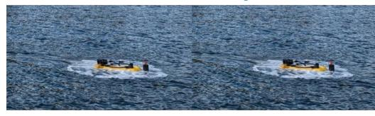
Greensea Systems, a leading provider of marine robotic software solutions, has successfully demonstrated untethered autonomy for remotely operated vehicles (ROVs). The company used a Defender ROV from VideoRay, equipped with batteries, an acoustic modem and the new OPENSEA Edge system, to showcase the untethered operation of an ROV at sea.
