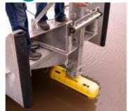
A quality control and filtering metric has been made available for EdgeTech and CARIS users. With their software release CARIS HIPS and SIPS supports the EdgeTech 6205's real time range and angle uncertainties which help significantly cut down on processing time. The EdgeTech 6205 is a Multi Phase Echo Sounder (MPES) that uses EdgeTech's bathymetric technology to provide an enhanced and fully integrated bathymetry and dual frequency side scan sonar system.
