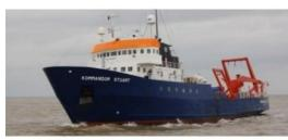
Horizon Geosciences announced the addition of a new vessel to its fleet, primed for work in the North Sea and West Africa. Kommandor Stuart is a DP1, multi-disciplinary, geophysical survey vessel with a proven track record in the North Sea and Arctic. Fitted with a high resolution 500m range multibeam echo sounder and a low frequency 3,000m range multibeam echo sounder as well as a full geophysical survey spread this vessel is available for site investigation and cable / pipeline route surveys.
