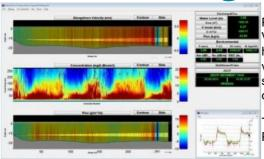
PDT-H is Aqua Vision's toolbox for the existing horizontal ADCP software suite, ViSea-H DAS. This toolbox lets the user quantify sediment concentrations and fluxes from horizontal ADCP data. PDT-H calculates suspended sediment fluxes by extrapolating the vertical concentration profile. The toolbox also lets the user post-process and optimise self-contained horizontal ADCP data with e.g. grain size distribution, calibration coefficients, etc.
