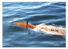
UK-based FUGRO Survey has ordered a HUGIN AUV to augment its existing fleet of survey vehicles. The new HUGIN 1000 AUV has depth rating of 3,000 metres and includes lithium polymer batteries. The batteries are packaged into modules, which are stacked in the centre section of the AUV.
