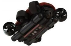
The 'Fusion' hybrid underwater vehicle is a real breakthrough. It uniquely combines autonomous underwater vehicle (AUV) and remotely operated vehicle (ROV) capabilities with diver navigation and propulsion into one system, thanks to Nortek's DVLs. Both the electronics and transducers are smaller and have a better form factor for the Fusion underwater vehicle. The higher frequency for
