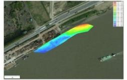
Eye4Software's hydrographic survey package, Hydromagic version 5.1, has been released. The software maps the bottom of a river, pond or ocean in 3D by using a (D)GPS or RTK positioning system combined with an echo sounder or fish finder. This version supports real-time calculation of the current tide level by using a RTK receiver connected to the PC.
