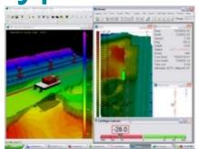
HYPACK 6.2A represents almost a year of improvements to the previous version HYPACK 6.2 and offers a turnkey surveying package for acquiring and processing bathymetry, ADCP, magnetometer, and side scan sonar data, charting tools for S-57 production.
