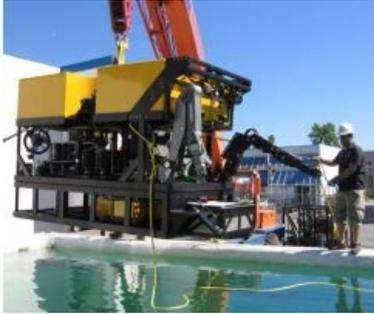
International Submarine Engineering Ltd has announced that it is pleased to deliver a new Remotely Operated Vehicle (ROV) and Tether Management System (TMS) to Fukada Salvage and Marine Works Co. Ltd. This HYSUB 100HP ROV is a multi-purpose vehicle that will be used for scientific and commercial purposes as well as inspecting and salvaging seafloor items.
