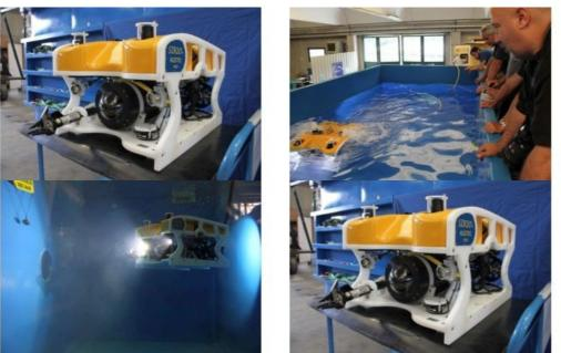
The ROV Sirio+ from Ageotec (Italy) is a small size system, based on the architecture of the popular inspection class Sirio, albeit with power delivered by four brushless thrusters of 450W each that make it suitable to operate in strong currents and in other tough situations. The three cameras allow technicians to inspect the artifacts at the front, at the back and also to observe the areas above the vehicle, all simultaneously.
