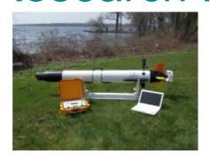
The Taiwan Ocean Research Institute (TORI) has acquired an Iver2 Autonomous Underwater Vehicle (AUV) to collect data for scientific research and improved environmental protection. The Iver2 EP42 vehicle capability includes side-scan sonar, acoustic current profiling, and a camera system along with both above and below surface communications.
