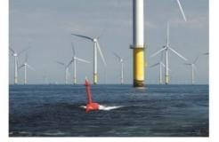
iXblue recently completed the bathymetric survey of the Saint Nazaire offshore wind farm using its DriX Uncrewed Surface Vehicle (USV). Relying on 4G and satellite communication, the operation – located 20km off the west coast of France – was remotely conducted by the iXblue teams of surveyors from their remote control centre in La Ciotat, south-east France.
