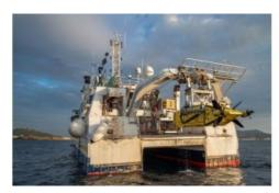
Ifremer, the French research institute for ocean science, has received its new synthetic aperture sonar (SAS) from iXblue. It will equip the institute's new 6,000m-rated autonomous underwater vehicle (AUV) dedicated to deep-sea exploration.
